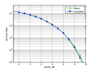
Fig.7. Gaussian Noise BER curve for wavelet source coding with OFDM
